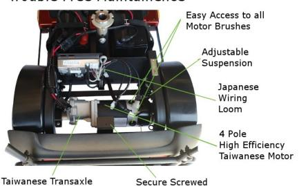
Secure Screwed Rear Shroud Mounting
